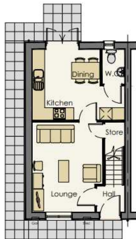
Ground Floor Plan 2B3P House Type 70sq.m
