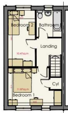
First Floor Plan 2B3P House Type 70sq.m
